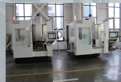
3 units DU500 with siemens one
